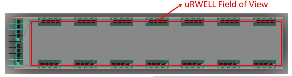
7 FEBs on each side + 2 FEBs on the service area Each FEB has 4 ASCIS (total 256ch), 1 data cable, 1 power cable Maximum length of FEB is ~160 mm (to be fit in the service area)
