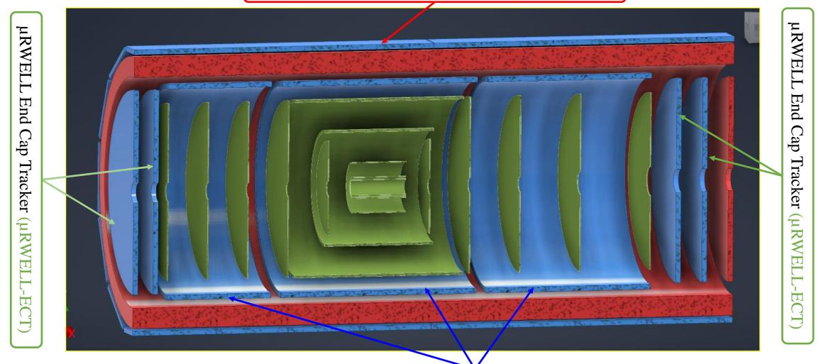
Inner Cyl Micromegas Barrel Layer (CyMBaL)
