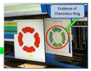
Pixel pattern & accumulated single photon XY-coordinates (offline)
