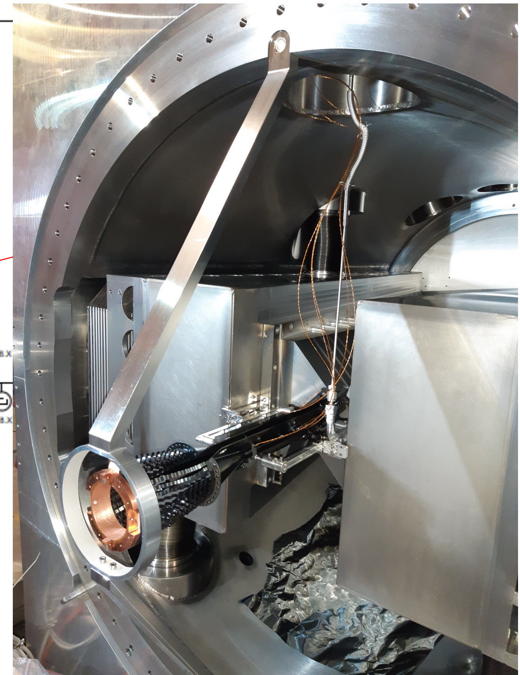
SMOG 2 Storage cell integration in the VELO vacuum tank
