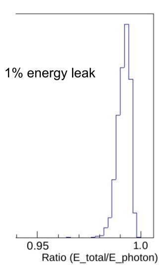
Mostly lateral energy leaks can be easily fixed by making a larger detector, but the highest average density of deposited energy reaches 12 MeV/cm³ per event which results in maximal absorbed dose of 550 Mrad for 100 fb<sup>-1</sup> of *ep* collisions
