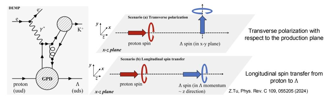
New  $\Lambda$  polarization measurement via deep exclusive meson production (DEMP):  $e + p \rightarrow e' + K^+ + \Lambda$  e',  $K^+$  can be measured within acceptance of central detector  $\Lambda$  (close to beam direction) decay particles can be measured using far-forward detectors
