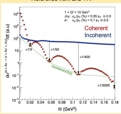
At position of third diffractive minimum, rejection factor for incoherent events better than 400:1 must be achievable (0.0025 % inefficiency)
