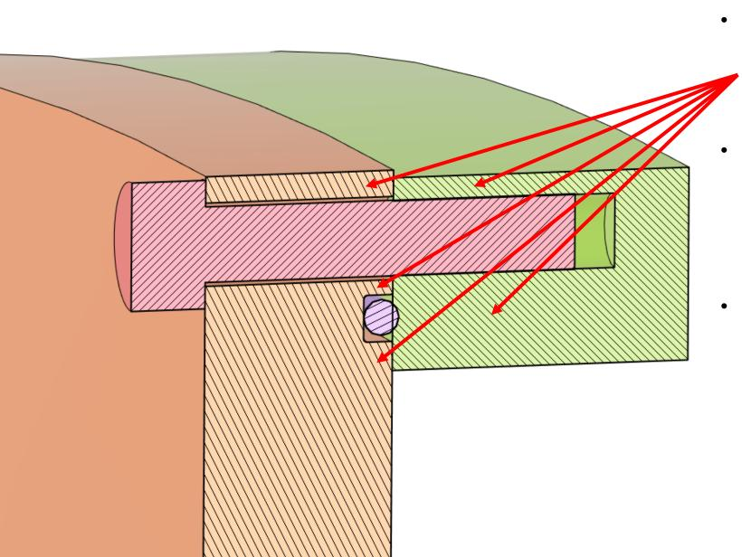
There is a need for a reasonable material thickness between the tapped hole, the o-ring groove and the edge of the parts for both the end ring (green) and the sensor plane (orange).
