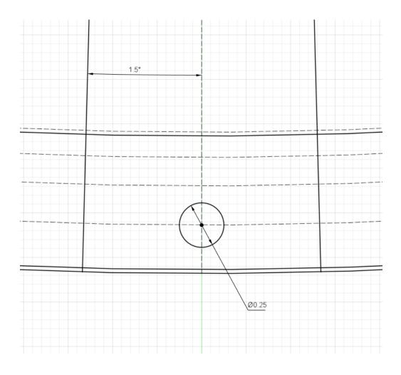
In full-gasketed joints uniformity of pressure on the gasket is important. To maintain adequate uniformity of pressure adjacent bolts should not be placed more than six nominal diameters apart on the bolt circle. To maintain wrench clearance, bolts should be placed at least three diameters apart. A rough rule for bolt spacing around a bolt circle is
