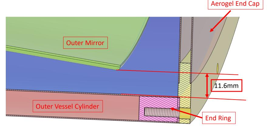
The current design (with a 3mm thick mirror) has about 11.6mm of clearance between the mirror and the inner CF wall. Moving from  $\frac{1}{2}$ " to  $\frac{3}{4}$ " thickness radially will take 6.35mm away from that, leaving us with 5.25mm of clearance on each side for installation.
