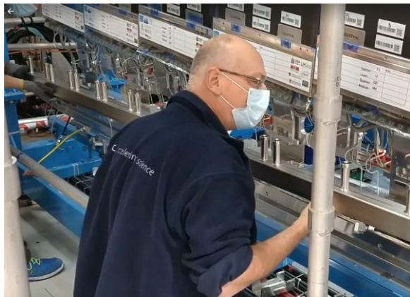
Replacing a defective cooling and vacuum manifold.
