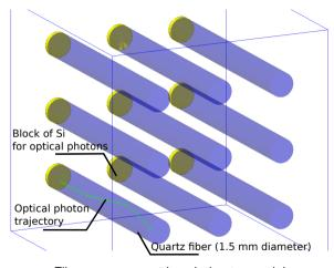
Fiber arrangement in calorimeter model
