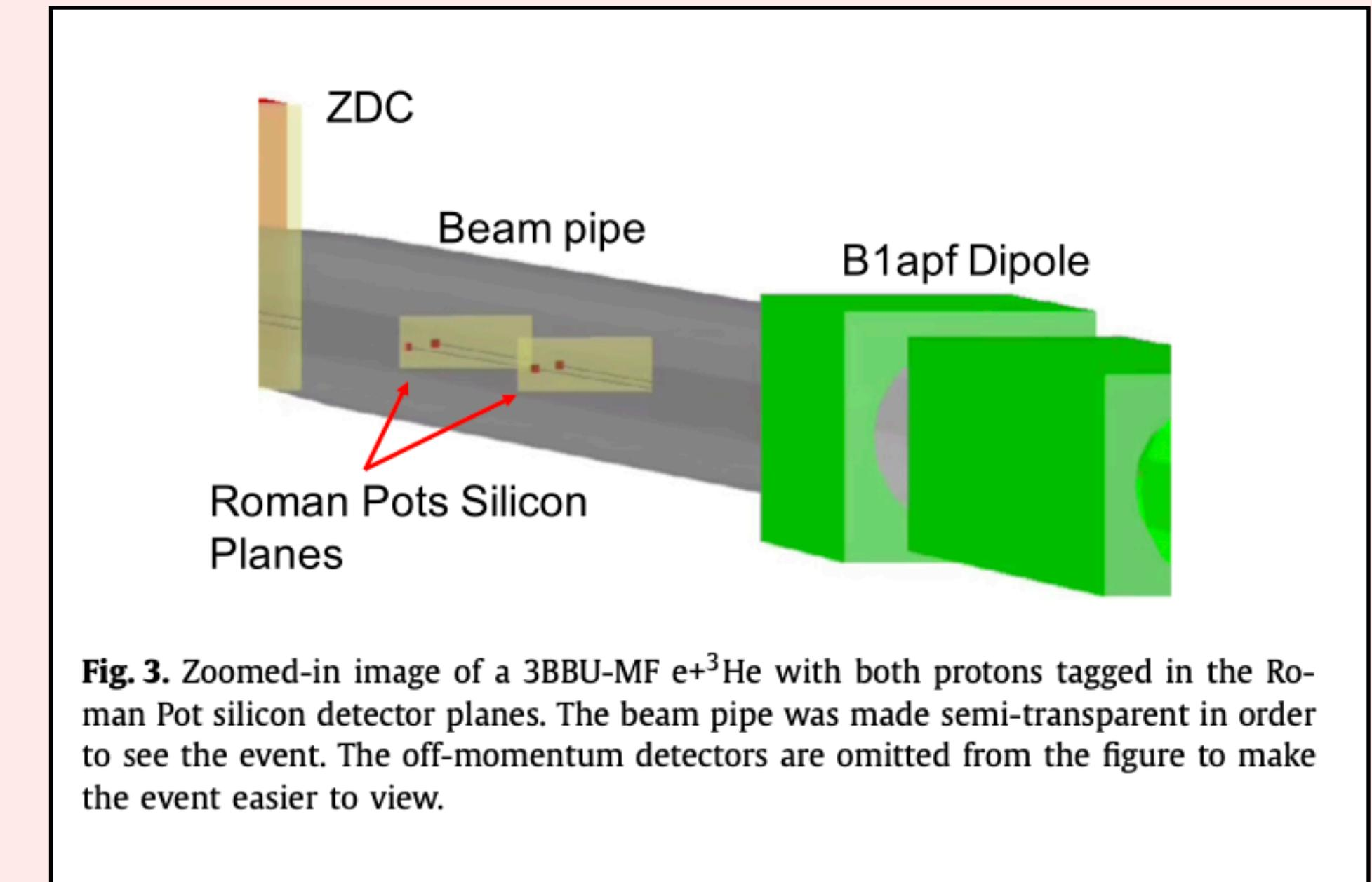
**Fig. 3.** Zoomed-in image of a 3BBU-MF  $e+{}^3\text{He}$  with both protons tagged in the Roman Pot silicon detector planes. The beam pipe was made semi-transparent in order to see the event. The off-momentum detectors are omitted from the figure to make the event easier to view.
