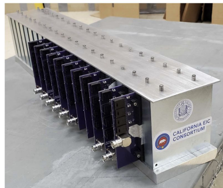
Figure 1. (Left): exploded view of prototype layer design. (Right): calorimeter insert prototype.
