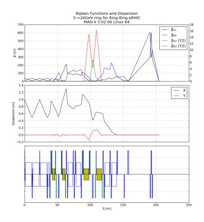
ullet Complete integrated design with dispersion suppressor, coupling compensation, low-eta section, and matching into arc
