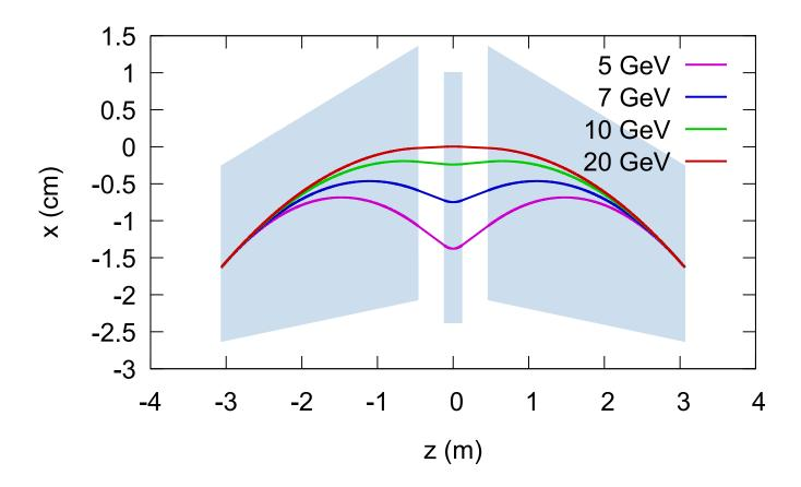
Short, sharp bends to increase damping decrement at low energies, thus allowing high electron beam-beam parameter  $\xi=0.1$
