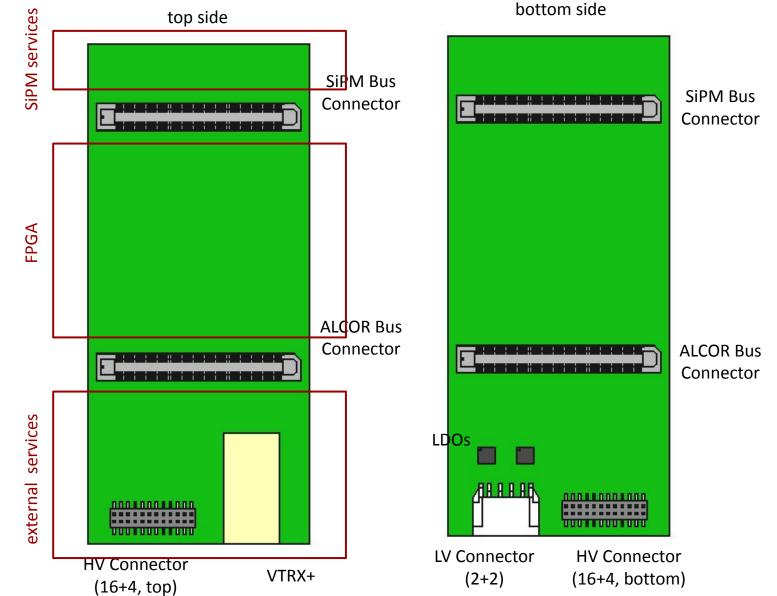
preferred clock to be received: 98.5 MHz, we aim ALCOR@396 MHz using SkyWOrks Si5236
