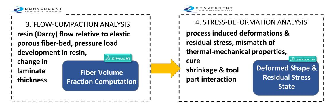
Material properties are updated at each solution step to account for the progression of cure and the subsequent change in thermal properties.
