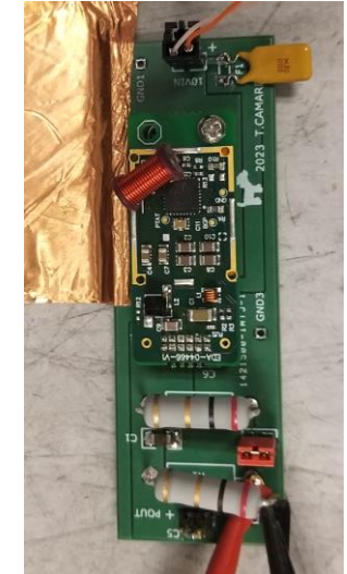
CERN bPOL12V 10W DC buck converter, high rad tolerant Availability? Need to purchase from stockpile
