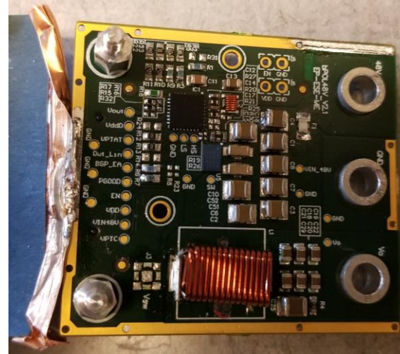
CERN bPOL48V2.1 , 1channel 100W DC buck converter, High rad tolerant
