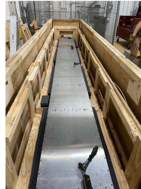
Test of finished new transportation crate with mock-up box
