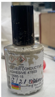
Ag epoxy to complete the electrical loop
