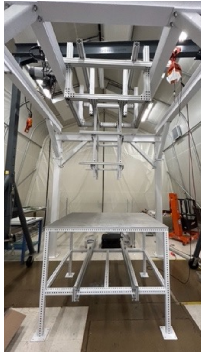
DIRC lab/CRT support structure at SBU
