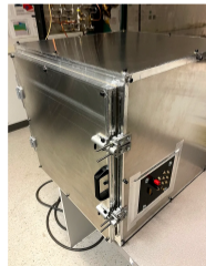
(a) Light-tight Faraday box with connector panel
