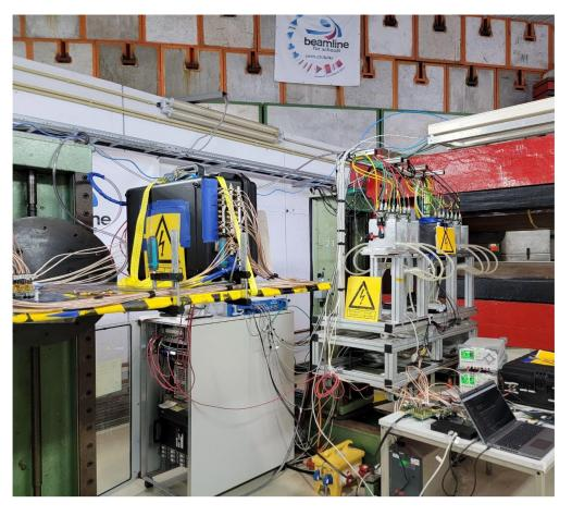
Current plan for this test beam: New HPK Sensors, EICROC0, FCFDv1 Beam Facility: telescope with 3 um resolution, trigger from scintillators
