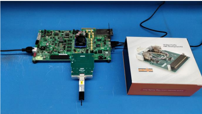
Samtec FireFly Test Setup with Fiber Loopback
