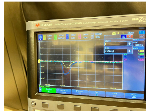
Example coincidence trigger from 2 paddles above and below the Baby BCal
