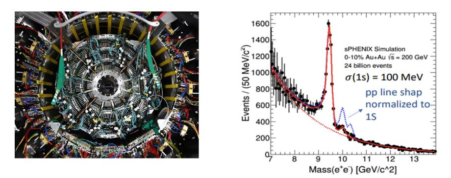
sPHENIX TPC provides invariant mass resolution better than 100 MeV/ $c^2$  for the Y di-electron channel.
