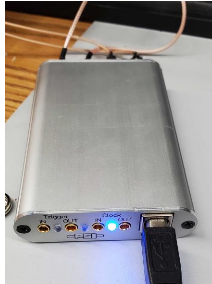
Full waveform digitizer (handheld)
