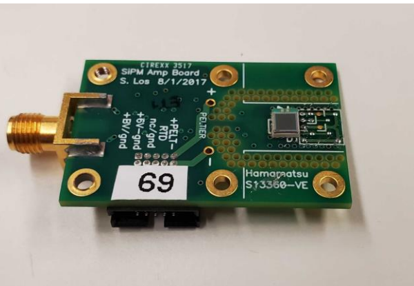
Single channel board with an amplifier built in – goes to scope
