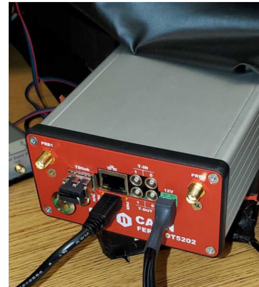
Bias and digitizer unit with 64 channels (handheld)
