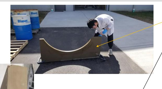
Application of densifier for the tooling board
