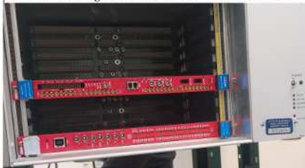
WEINER VME crate: CAEN V1718 controller board CAEN V1742 Digitizer board with 32 readout channels
