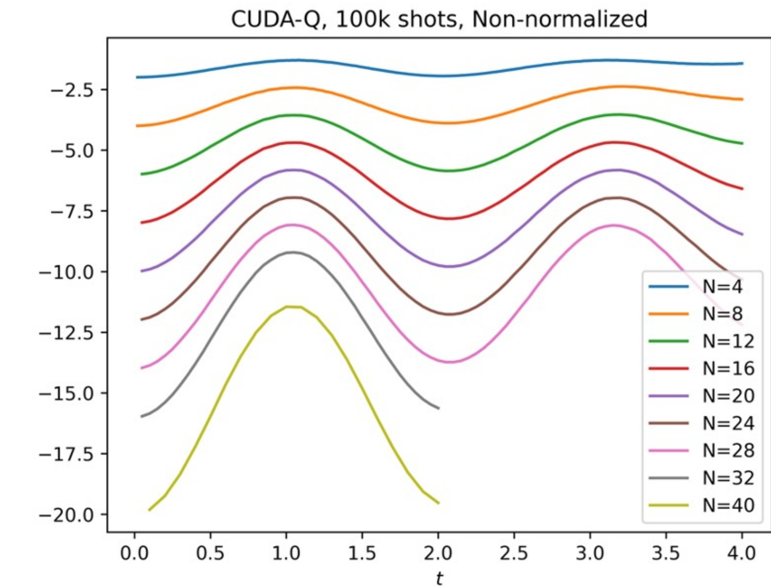
Higher qubit runs enabled by CUDA Quantum help in improving accuracy in determining peak values
