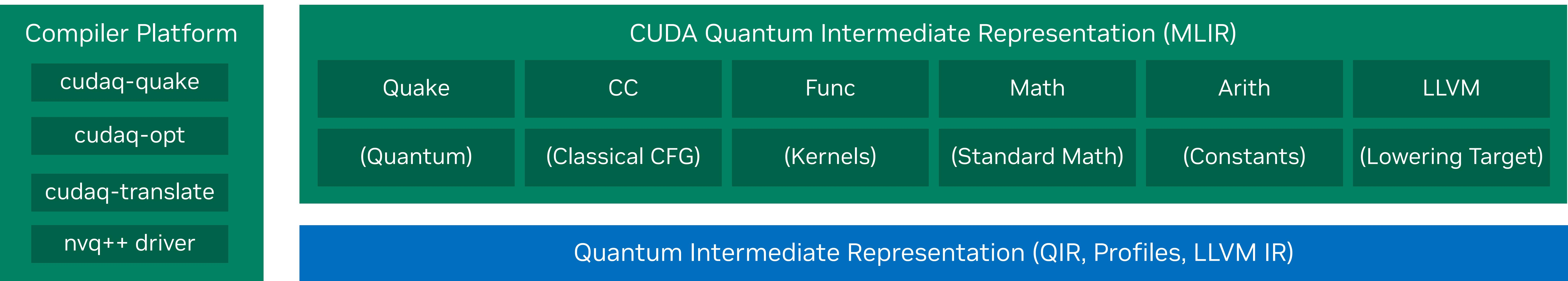
CUDA Quantum provides a collection of tools that enables the compilation of Kernel representations to external representations like the QIR.
