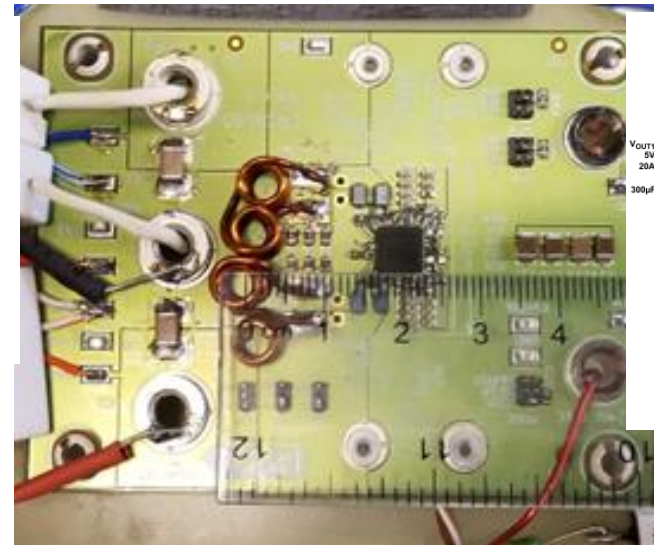
LTC 7890 (GaN Controller) evaluation board (replacement candidate for CERN bPOL48V controller for lesser harsh rad environments)
