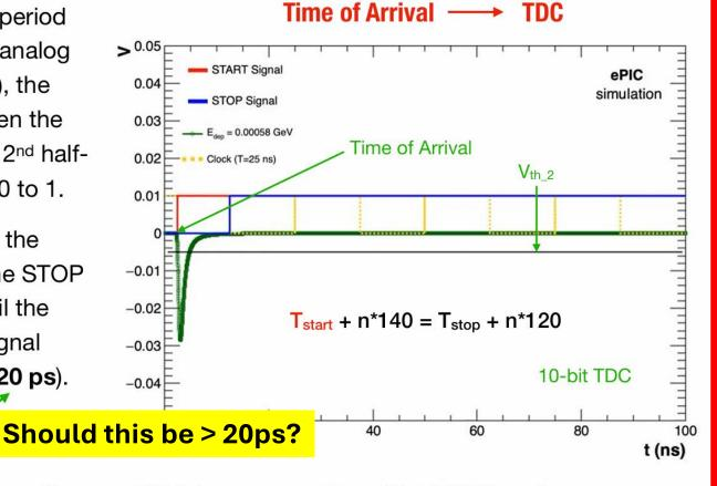
• The number of times the signals move  $(1 \le n \le 1024)$  is converted to a 10-bit TDC code.
