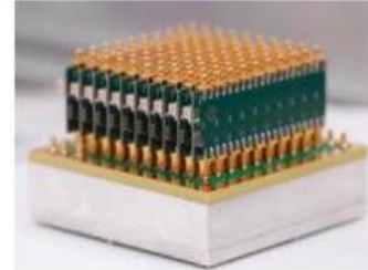
Multi-channel custom-made pre-amplifier (M. Kovacic, U. of Zagreb)
