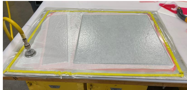
Plate layups for outer plate and interstitial beams
