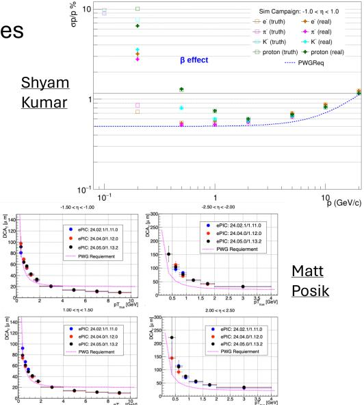
Possible impact due to mismatch between Acts material map and Geant-level geometry. Need a better way to ensure consistency when running simulations.
