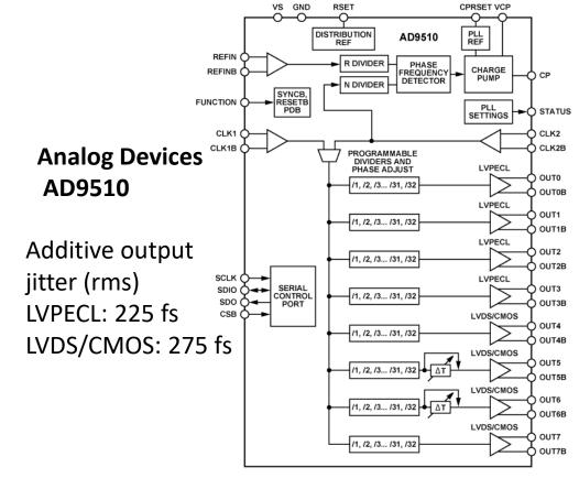
Used on the Trigger Interface modules to generate **SYNCHRONIZED** /2, /4, /6 and /8 lower frequency clocks
