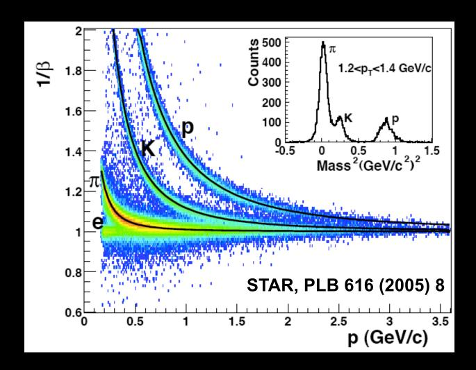
TPC and TOF combined provide clean particle identification.
