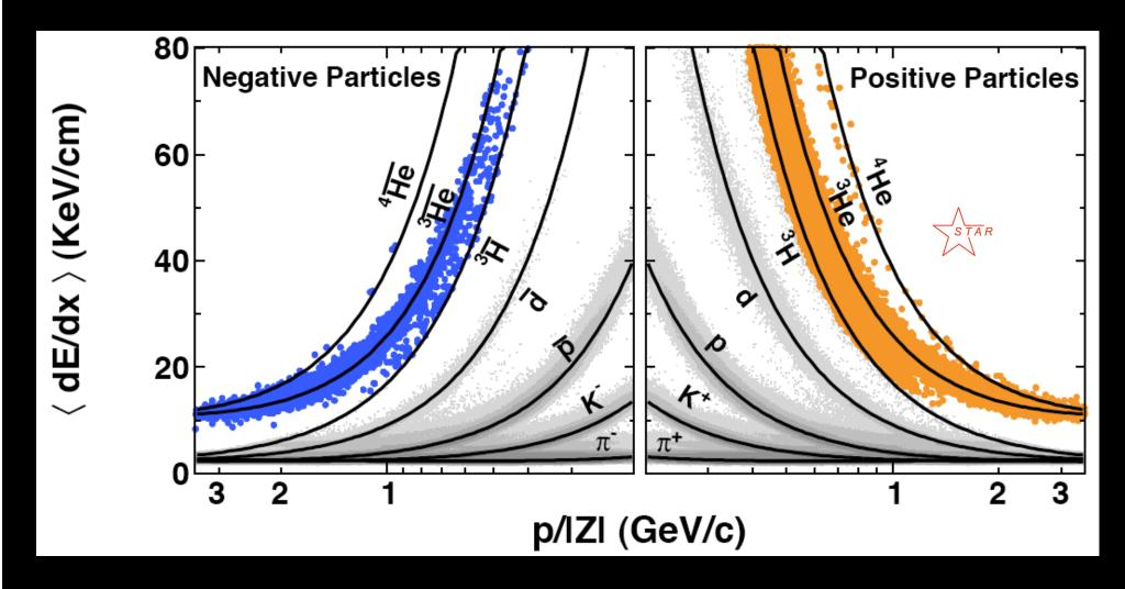
HLT has processing power to do rudimentary event reconstruction in real time, allowing events with a |Z| = 2 track to be tagged and fast-tracked via the normal offline calibration & reconstruction chain.
