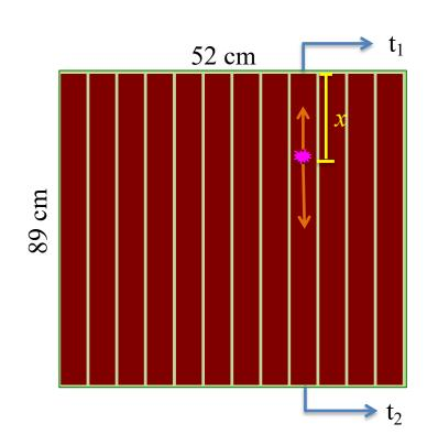
HW: given that the time signals for a particle hitting a strip of length L are  $t_1$  and  $t_2$ , and the signal travel velocity in the strip is v, what is the time and position of the hit?
