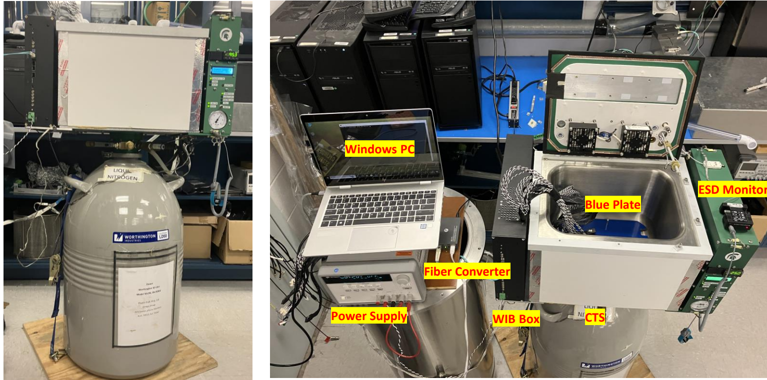
QC Test Setup Hardware
