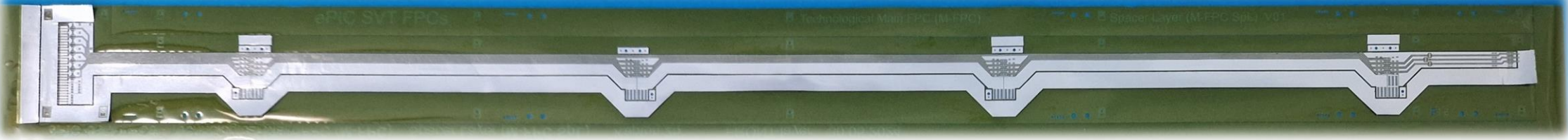
Stage 2: 3-layered FPC (2-layered FPC + GND Layer)
