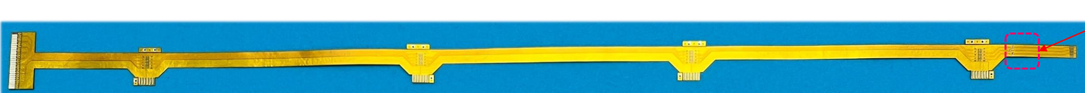
Stage 3.2: 4-layered FPC (4-layered FPC +SMDs)
