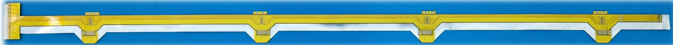
Stage 3.2: 4-layered FPC (4-layered FPC +SMDs)
