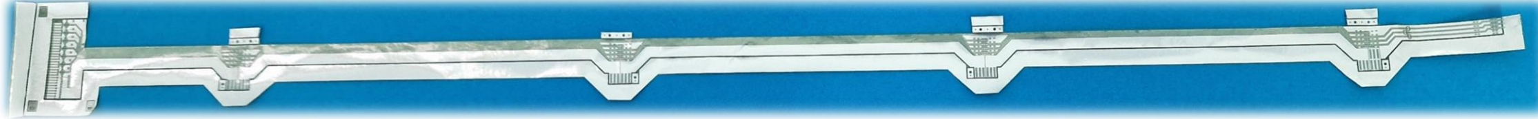
Stage 3.1: 4-layered FPC (3-layered FPC + Cover Layer+SMDs)
