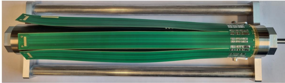
FPC of layer 0 assembled on a mandrel.
