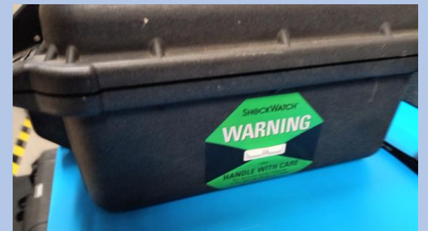
HRPPD-25 case with shock sensor
