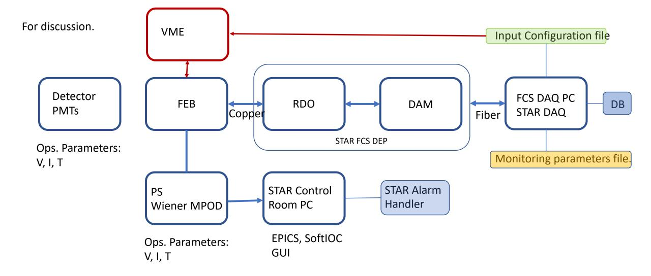
Independent form STAR DAQ way to configure and take data via slow control (VME based hardware, TCL script) (pedestals, noise, pulser, LED runs) was very useful to maintain and operate BEMC. Parallel method of controlling FEEs independently from any other sub-systems at STAR.
