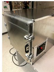
(a) Light-tight Faraday box with connector panel
