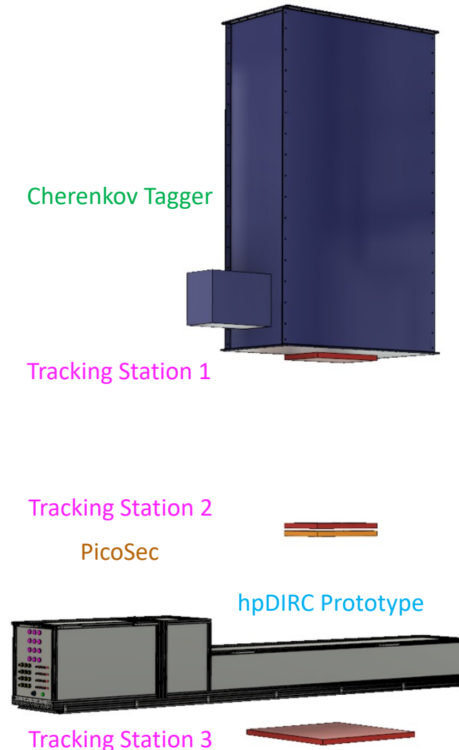
CRT setup CAD schematic
