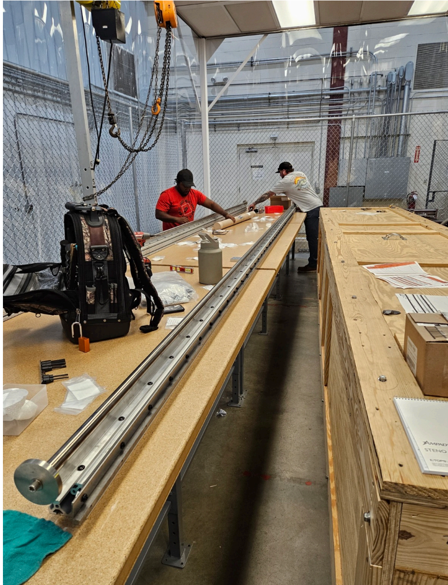
Rails for CNC under construction
