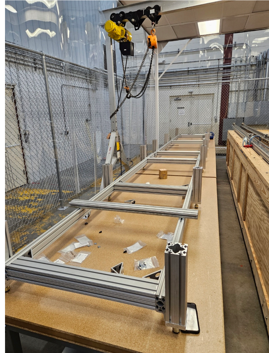
Support structure to level the bar box
