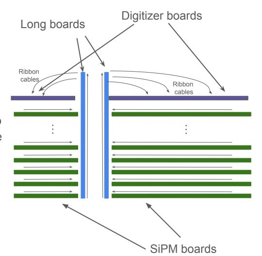
Long board for transfer to readout (x4)
