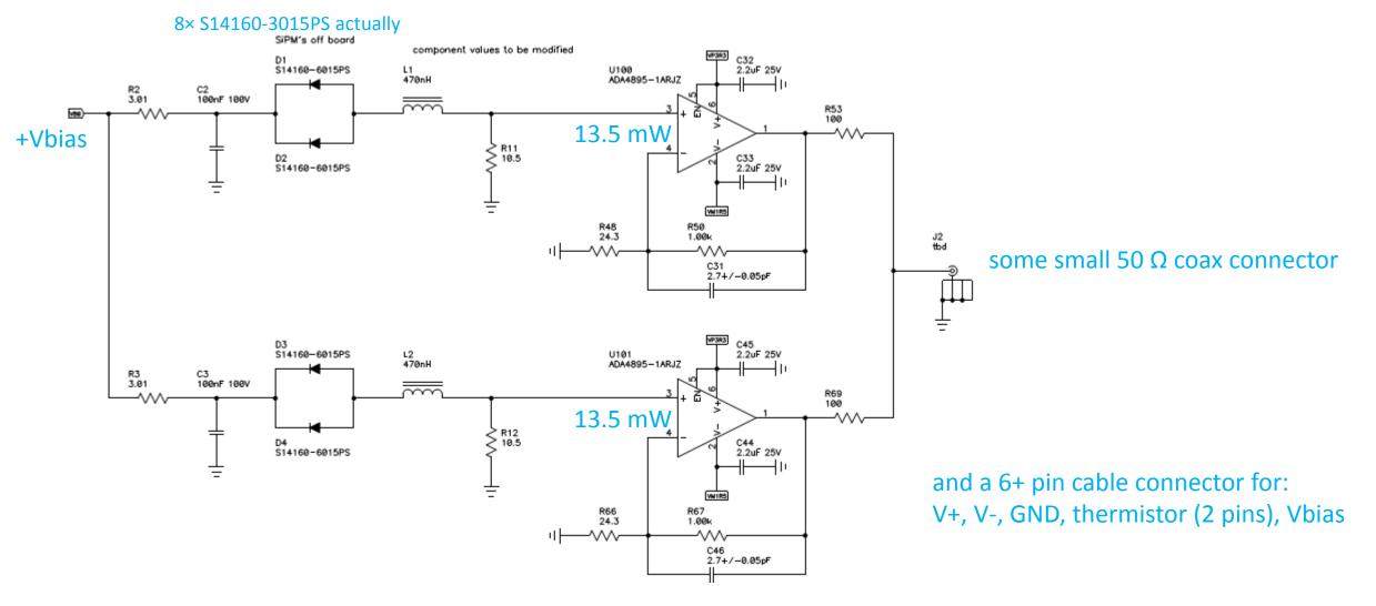
the signal output from this should be compatible with other waveform ADC's, e.g. JLab fADC250
