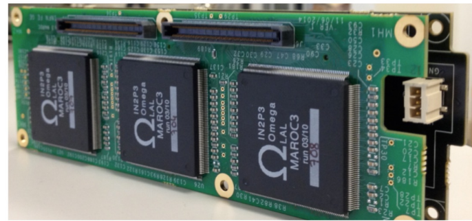
ASIC board produced for the RICH detector for CLAS12 with MAROC chips installed
