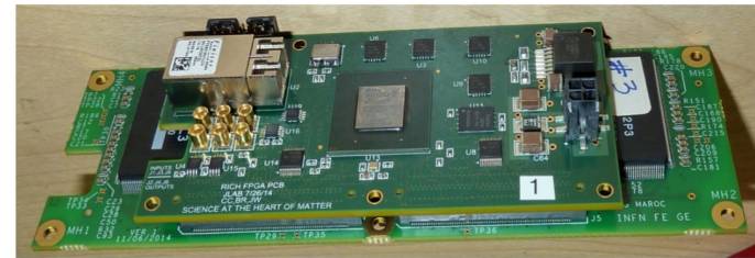
FPGA Screenshot for the RICH detector for CLAS12 with ASIC board attached
