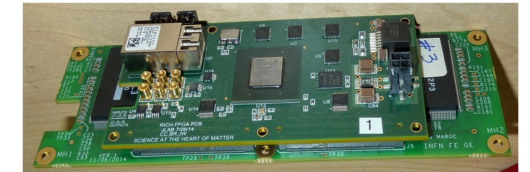
FPGA Screenshot for the RICH detector for CLAS12 with ASIC board attached
