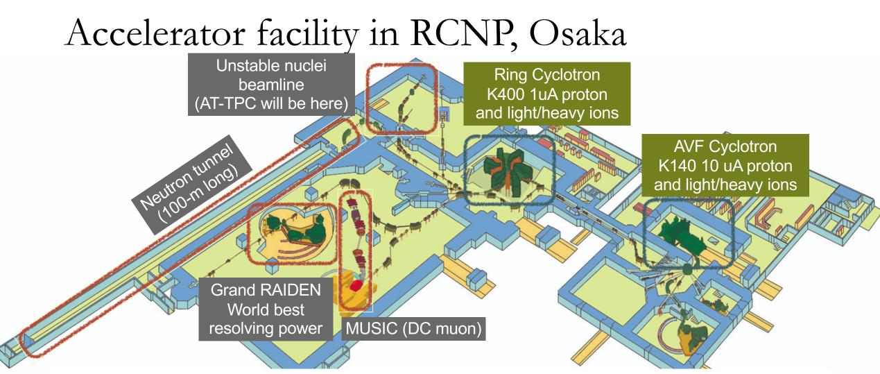
Ion beams (protons, deuterons, and heavy ions), continuous muon beams, and white neutrons available Used not only in basic physics, but also in medicine (RI drugs), archaeology, engineering, etc.
