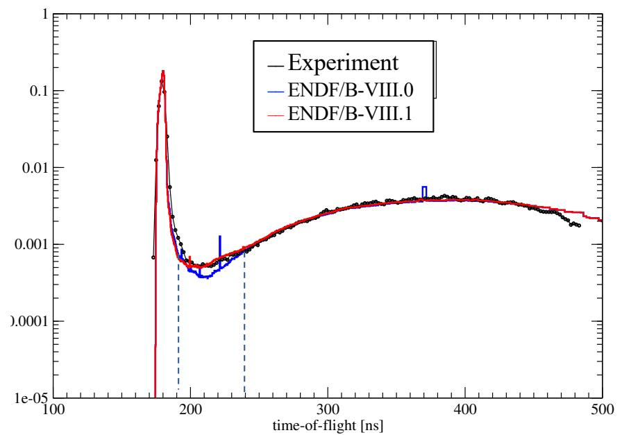
The Pu239 spectrum simulated with e81 shows improved agreement with experiment in the 190-240ns. Slight improvement for U235.
