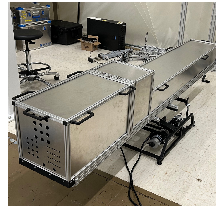
hpDIRC prototype on motion control stage
